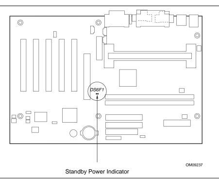
Figure 6. Location of Standby Power Indicator LED
